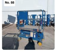
Serial Number: 19432413A Weight: 342kg Payload: 250kg No. Pax + alowance: 1 pax(80kg) +170kg Working Height: 5100mm Max. Manual Force: 200N Indoor use only CE Standard
