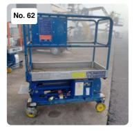
Serial Number: 16944211A Weight: 342kg Payload: 250kg No. Personas + alowance: 1 pax(80kg) +170kg Working Height: 5100mm Max. Manual Force: 200N Indoor use only CE Standard IMPORTANT: The customer is responsible for all the loading related to the equipment. Dimensions and weights are approximate.
