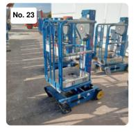
Serial Number: 2215012G Weight: 150g Payload: 150kg No. pax + alowance: 1 pax Working Height: 3500mm Max. Manual Force: 200N Indoor use only CE Standard
