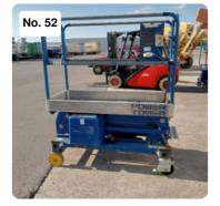
Serial Number: 1462510A Weight: 342kg Payload: 250kg No. Pax + alowance: 1 pax(80kg) +170kg Working Height: 5100mm Max. Manual Force: 200N Indoor use only CE Standard
