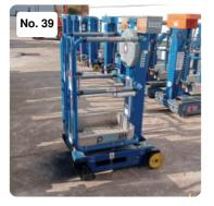
Serial Number: 4420613G Weight: 150g Payload: 150kg No. Personas + alowance: 1 pax Working Height: 3500mm Max. Manual Force: 200N Indoor use only CE Standard IMPORTANT: The customer is responsible for all the loading related to the equipment. Dimensions and weights are approximate.
