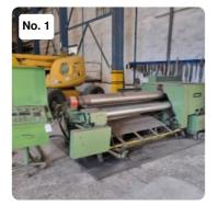
Round bending machine Serial number 4475 With 4 bending rollers: · 2 rollers with 220 mm diameter · 2 rollers with 180 mm diameter Rollers length: 2050 mm Maximum bending capacity: 2000 x 10/5 With output table of 1600 x 2260 mm Working hours according to counter: 4443 h 380V connection
