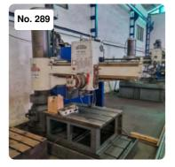
Serial number 2362 11405 Work table measurements: 1250 x 900 x 500 mm Working speed from 24 to 1210 Rpm Approximate horizontal travel: 1300 mm Approximate vertical travel: 900 mm Motor disassembled !!
