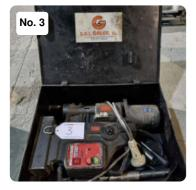
Heavy-duty drilling machine Serial number 040101711429 Power consumption 1800 W 4 working speeds: 85 - 135 - 160 - 250 Rpm Maximum milling capacity: 111 mm diameter Maximum drilling capacity: 47 mm diameter Maximum countersinking capacity: 63 mm diameter Max tap size: M30 Stroke: 230 mm Maximum cutting depth: 76 mm Accessories included
