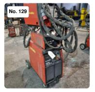
Serial number H17315973 Usage factor at 40%: 400 A Usage factor at 60%: 326 A Usage factor at 100%: 255 A Current regulation range: 30-400 A Three-phase connection CASTOLIN DERBY RE 230 wire feeding units With wheels for easy transport
