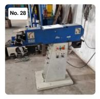
Serial number 392-19-0151 Motor power: 2.5-3.3 kW Working speed: 1400 - 2800 Rpm Belt speed: 15 - 30 m/sec Diameter of the piece to be sanded: 20 - 76 mm Adjustable angle from 0 to 90° Sanding band: 2000 x 100 mm Connection: 400V CE Standards
