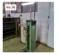
Point welding equipment Serial number 66264 Power at 50% F.M.: 18 kVA Maximum thickness when welding: 4 + 4 mm Rod capacity (diameter): 10 + 10 mm Standard neckgoose: 380 mm Distance between arms: 220 mm Electrode holder diameter: 20 mm Cooling water flow: 250 l/h Current regulation range: 100-150 A
