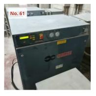
Screw compressor Serial number 1052567 Power 22 kW Maximum working pressure: 8 bar Flow rate: 216 m3/h Working hours according to counter: 20568 h CE Standards
