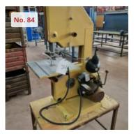
Band saw Serial number 17219-03 Worktable size: 375 x 375 mm 45° tiltable table Pulleys diameter: 320 mm Saw width: 9 mm Working speed: 300-700 m/min With LED lighting system for better visibility Support table included
