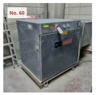
Screw compressor Serial number 1002059 Power 22 kW Maximum working pressure: 8 bar Flow rate: 216 m3/h Working hours according to counter: 24783 h CE Standards
