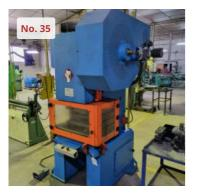
Eccentric press Model: T 50 CE Serial number 11287 Nominal force: 500 kN Nominal stroke: 3 mm Adjustable stroke: 12 - 110 mm Stop time: 121ms Safety distance: 194 mm Cycles per minute: 140 Table measurements: 750 x 440 mm Total installed power: 4.05 kW
