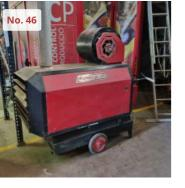
Industrial heater Serial number 8610 Rated power: 120.000 Kcal/h Power: 139 kW Air flow: 7.800 m3/h Ventilation power: 1.5 kW With wheels for easy transport
